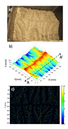
**Figure 2.** Photograph (a) and the DEM (b) of the evolved landscape at the steady state obtained from the eXperimental Landscape Evolution (XLE) facility at the St. Anthony Falls laboratory of University of Minnesota. The river network at the steady state extracted from the DEM at steady state is shown in (c) with the color bar
